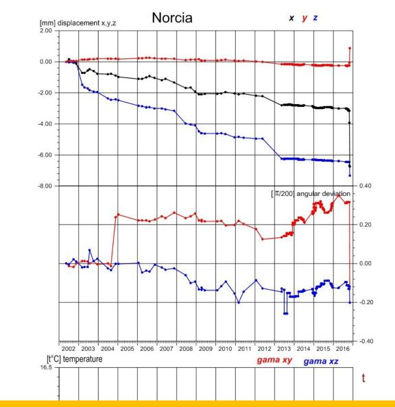
**Cumulative curve of fault slip recorded across Norcia Fault in Central Appenines**
