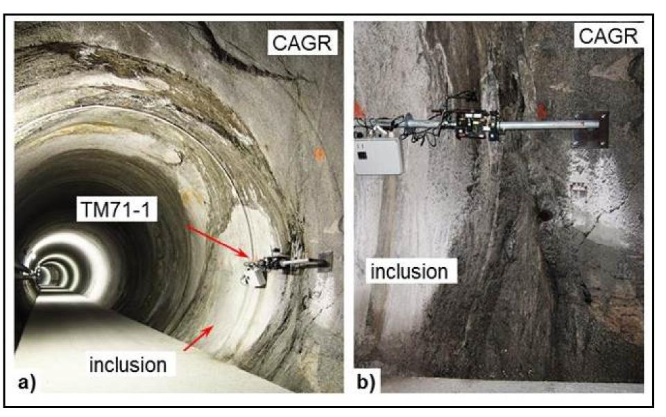
Type of TM71 installation:Grimsel Test Site (NAGRA, Switzerland),about 350 m under surface, LArge Scale MOnitoring project 2014 - 2018
